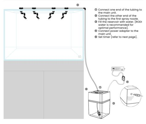
**Connecting nozzles:** Insert tubing into each nozzle and engage safety lock. Pull back gently to ensure the connection is secure.
